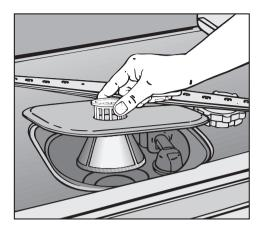
Lift the filter out of the machine. Remove any solid particles and rinse under running water. Scrub with a nylon brush if necessary.
